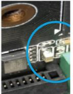
Components are sheared off when the card is inserted into a workstation slot that meets specification
