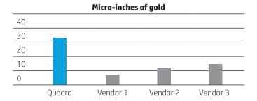
The customer cards are below 15 micro-inches and could experience early lifetime failures
